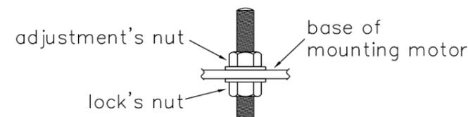
Until the belt works well in fitting the pulley, it takes several days. So, you run the machine a few days later, adjust the belt's tension again.
